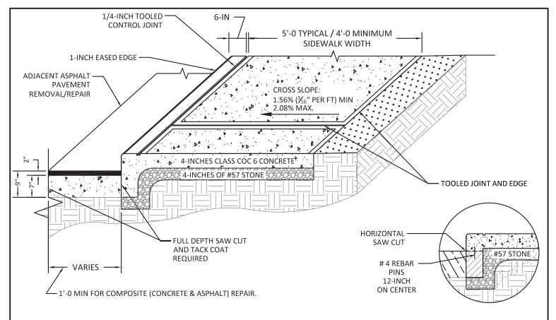
ISOLATED REPAIR DETAIL
