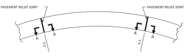
RELIEF JOINT DETAIL FOR PAVEMENT SECTIONS WITH C/L RADII TO 500' AND DELTAS ( $\triangle$ ) GREATER THAN 50°
