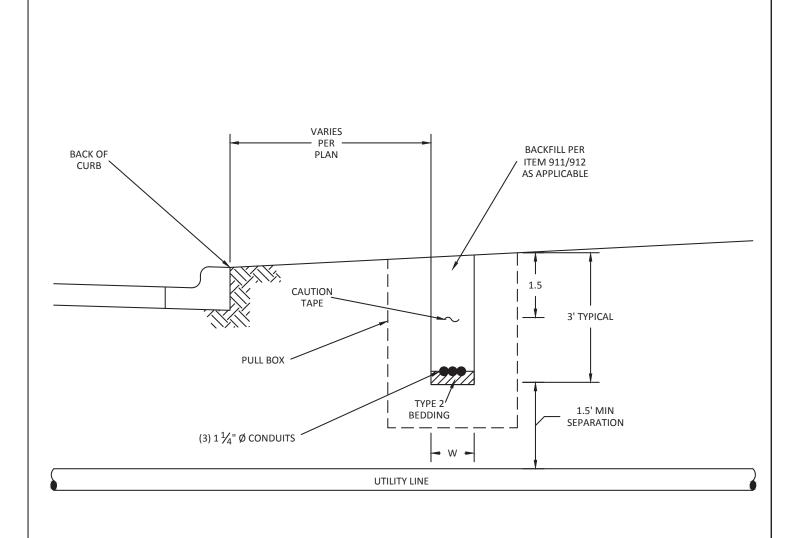
NOTE: TRENCH WIDTH 'W' MUST BE WIDE ENOUGH TO ACCOMMODATE AVAILABLE BACKFILL COMPACTION EQUIPMENT TO MEET COMPACTION REQUIREMENTS.
